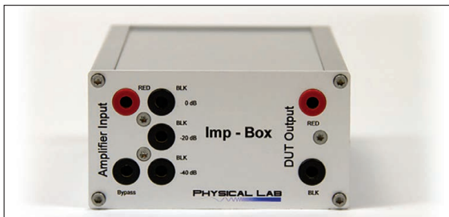
Photo 2: I used the Physical Lab IMP Box, which was provided to Voice Coil courtesy of Physical Lab, to take current and voltage measurements.
